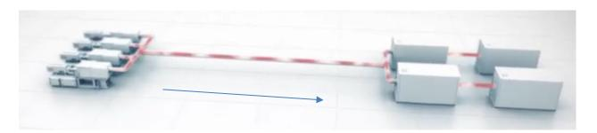
Air compressors directly supply machines on demand using minimum storage units in between, mainly in order to protect the compressors from frequent shutdown. This is a highly inefficient and costly methodology.
